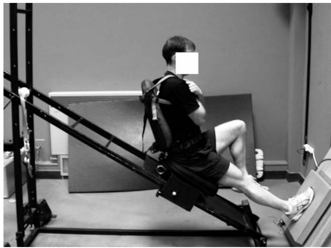
**FIGURE 1.** Photograph of the setup of the sledge and force platform apparatus showing a subject about to perform a single-legged CMJ.
